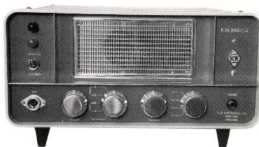
Fig.2: Ben G4BXD recently discovered this unusual transceiver, the KW2000CA, a 'special' four-channel crystal-controlled version of the well known Amateur Radio KW2000 transceiver (see text).
